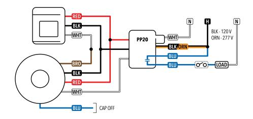
LOW VOLTAGE ON/OFF & AUTOMATIC DIMMING PHOTOCONTROL W/ LOW VOLTAGE OCCUPANCY SENSORS
