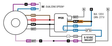
\*Wire VIO to additional 0-10 VDC Ballast & wire BLU to an Additional PP20
