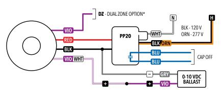
\*Wire to an additional 0-10 VDC Ballast
