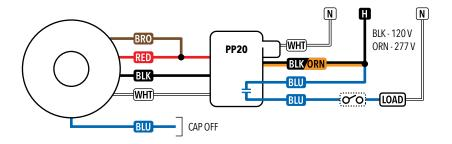
LOW VOLTAGE AUTOMATIC DIMMING PHOTOCONTROLS
